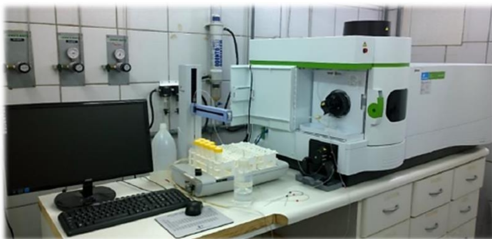
Figure 4: Perkin Elmer ICP-OES equipment, model Optima 8300 with autosampler model S10 used for trace element determinations.
